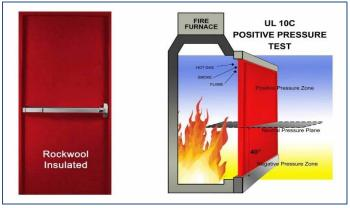
A fire door is a door with a fireresistance rating (sometimes referred to as a fire protection rating for closures) used as part of a passive fire protection system to reduce the spread of fire and smoke between separate compartments of a structure and to enable safe egress from a building or structure or ship.
